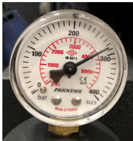
1.9) The manometer should be at 300 bars.
